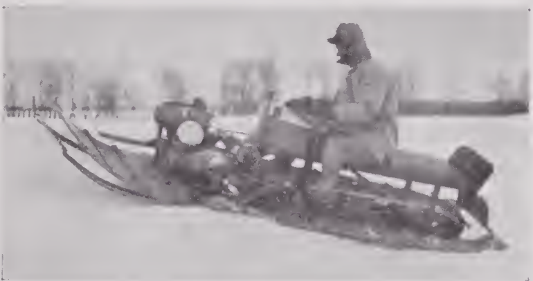
FIGURE 3. Eliason toboggan, driven by single 10-inch track, forced downwards by spring reacting against dead weight of vehicle.
